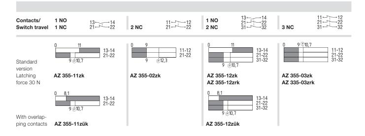
**Notes** Inserted position of actuator = 0 in switch travel diagrams.
